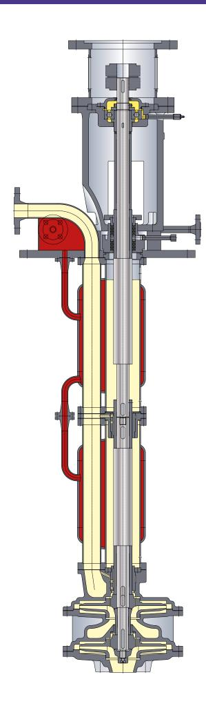
The compact construction is suited to fit in small container openings. Thanks to the grease-lubricated roller bearing system above the mounting flange, even high temperature applications can be handled. The casing design minimizes pressure losses and thus operates in a highly efficient way.
