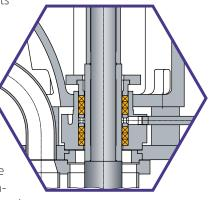
thus ensures a low level of sleeve bearing wear during constant pump operation. Costly oil lubrications or additional cooling which have an impact on safety are not necessary. The pump is fitted with a heating jacket to maintain the pumped sulphur at a constant temperature and, consequently, unchanged viscosity. Each individual segment of the pipe string is encased in its own heating jacket in this respect.
