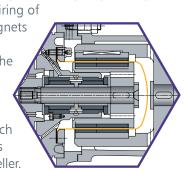
The external or atmosphere side magnet system is separated from the internal product side magnetic system by a spacer can made of non-magnetic material. The torque needed to drive the impeller is transmitted exclusively by magnetic forces which act through the spacer can. The pump it is thus hermetically sealed.
