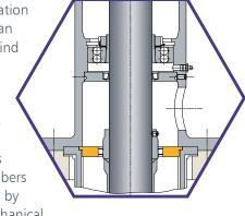
seals with a lip ring. This sealing principle is also applied as stationary sealing for hydrodynamic shaft seals.
