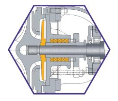
dro-dynamically from the pump and inlet pressure. The medium is kept away from the shaft gland.
